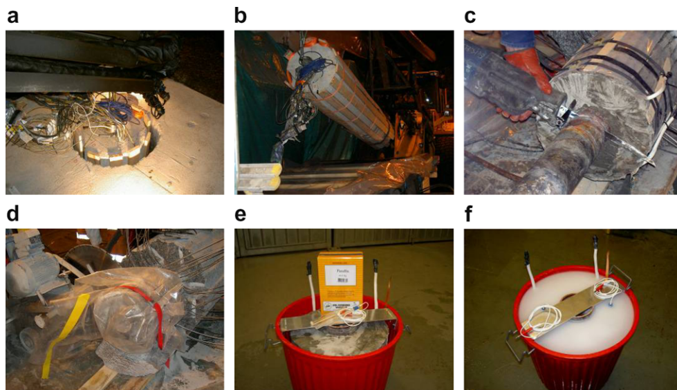
Fig. 8. Retrieval of the pre-exposed copper electrodes in January 2006. (a–b) Lift-up of the test parcel with surrounding rock, (c–d) cutting off the bentonite test package after removal of surrounding rock, and (e–f) moulding the bentonite test package in paraffin.
